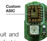
The ASIC contains power circuit and this helps to avoid defects by electric damage from the power line.
