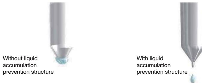
Liquid leakage detection
