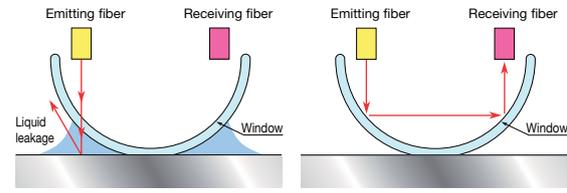
Light from the emitting fiber is reflected by the liquid leakage and not detected by the receiving fiber.
