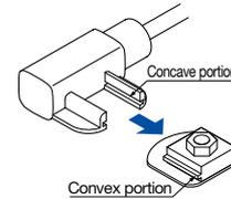
**Mounting pipe-mounted liquid level detection fibers (NF-TF01)**
