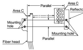
**Mounting liquid leakage detection fibers (NF-DW02)**
