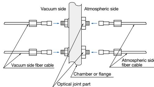
Leakage amount:  $1.33 \times 10^{-10}$  Pa·m<sup>3</sup>/s [He] or less
