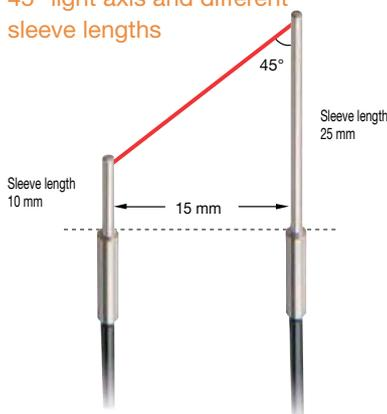
Angle detection using conventional fiber units
