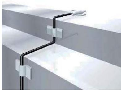
Extra space is unnecessary as the bending radius is 1 mm. No more worrying about snagging.
