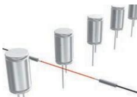
Presence of capacitor leads
